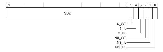
Figure 3-55 Cache Behavior Override Register format
