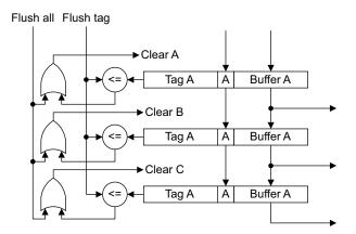
Figure 11-6 Queue flushing
