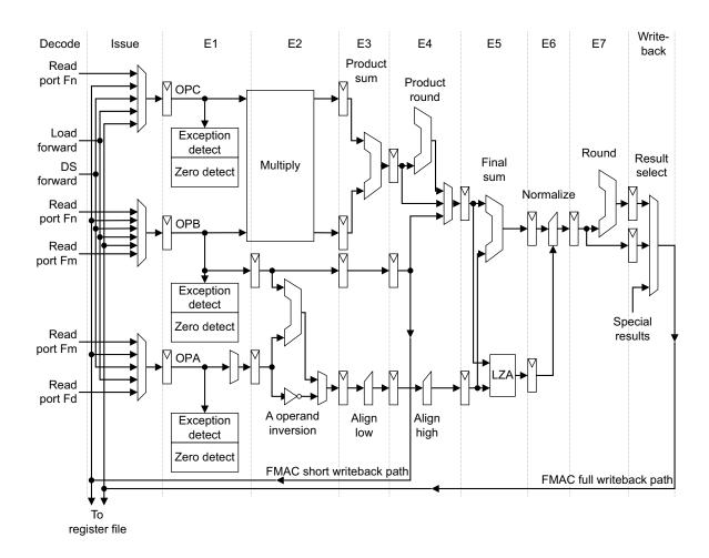
Figure 18-1 FMAC pipeline
