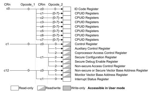
Figure 3-1 System control and configuration registers
