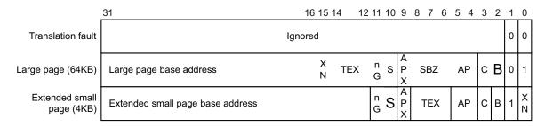
Figure 6-8 ARMv6 second-level descriptor format
