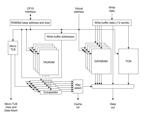
Figure 7-1 Level one cache block diagram
