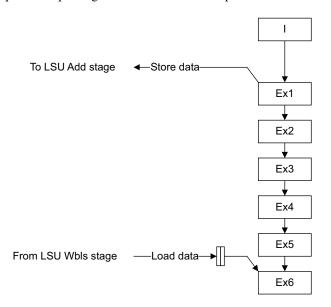
Figure 11-8 Coprocessor data transfer
