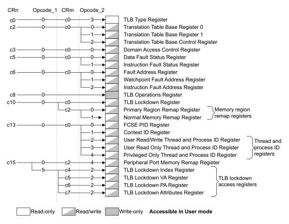
Figure 3-2 MMU control and configuration registers
