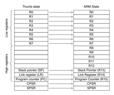
Figure 2-9 ARM state and Thumb state registers relationship
