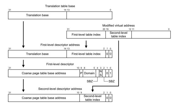
Figure 6-13 Generating a second-level page table address
