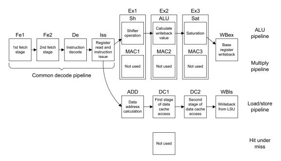
Figure 1-6 Progression of an LDR/STR operation
