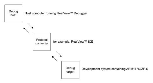
Figure 13-1 Typical debug system
