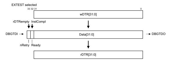
Figure 14-10 Scan chain 5 bit order, EXTEST selected
