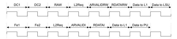
Figure 9-2 Read latency with no IEM
