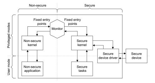
Figure 2-1 Secure and Non-secure worlds
