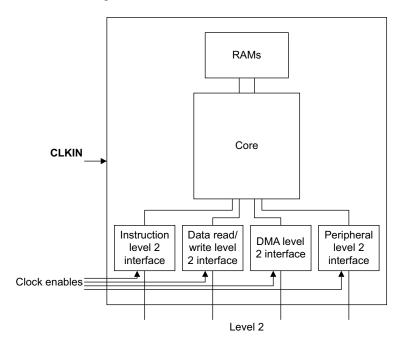
Figure 9-1 Processor clocks with no IEM
