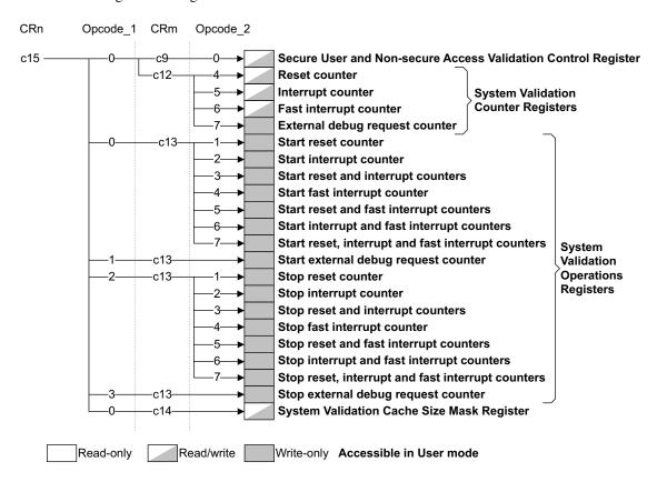
Figure 3-8 System validation registers
