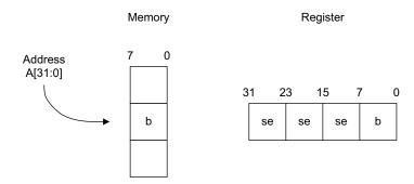
Figure 4-2 Load signed byte
