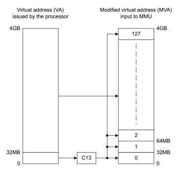
Figure 3-69 Address mapping with the FCSE PID Register
