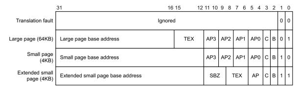
Figure 6-5 Backwards-compatible second-level descriptor format
