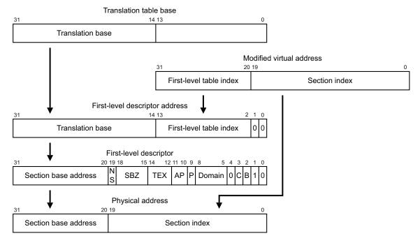
Figure 6-12 Translation for a 1MB section, backwards-compatible format
