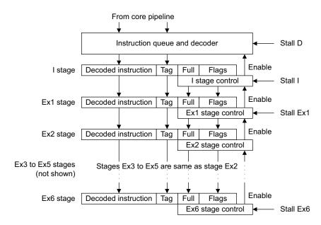
Figure 11-3 Coprocessor pipeline
