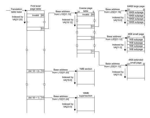
Figure 6-6 Backwards-compatible section, supersection, and page translation
