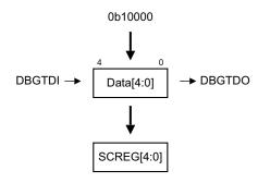
Figure 14-6 Scan chain select register bit order
