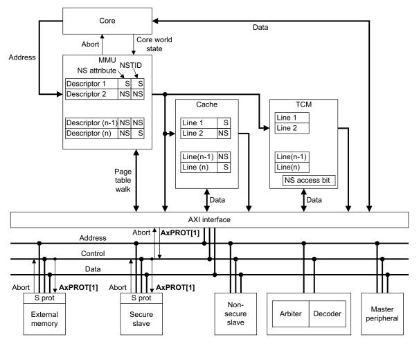
Figure 2-2 Memory in the Secure and Non-secure worlds
