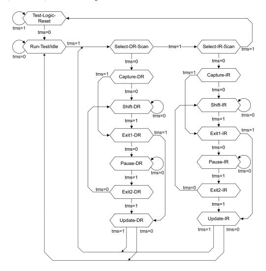
Figure 14-1 JTAG DBGTAP state machine diagram<sup>1</sup>
