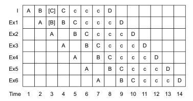
Figure 11-9 Instruction iteration for loads
