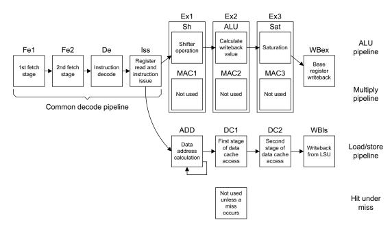
Figure 1-7 Progression of an LDM/STM operation
