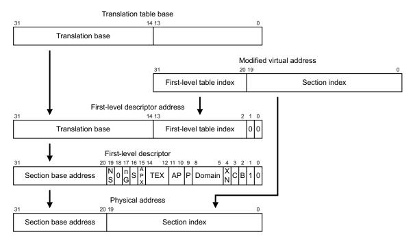
Figure 6-11 Translation for a 1MB section, ARMv6 format
