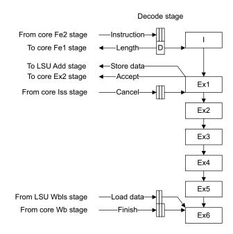
Figure 11-2 Coprocessor pipeline and queues
