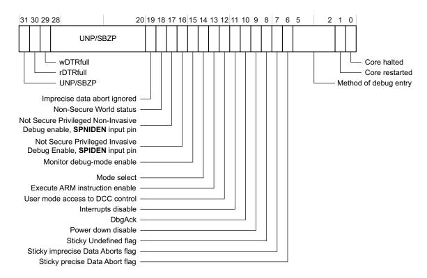
Figure 13-3 Debug Status and Control Register format
