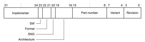
Figure 20-5 Floating-Point System ID Register
