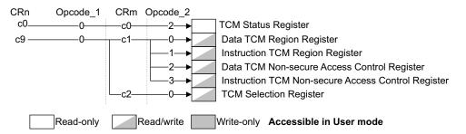
Figure 3-4 TCM control and configuration registers
