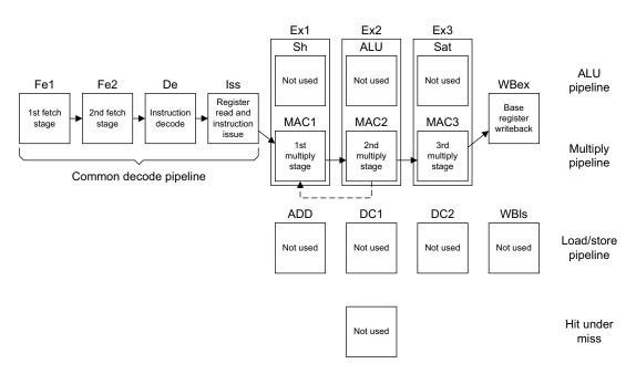
Figure 1-5 Typical multiply operation
