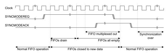
Figure 9-4 Processor synchronization with IEM
