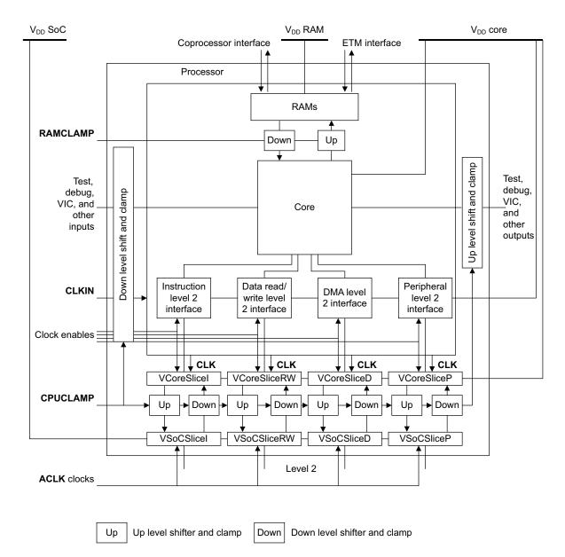
Figure 10-1 IEM structure
