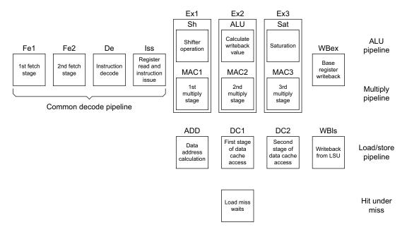
Figure 1-3 Typical operations in pipeline stages
