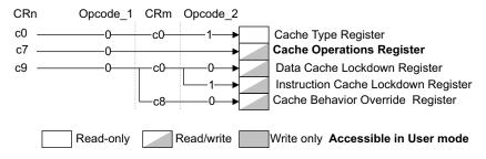
Figure 3-3 Cache control and configuration registers
