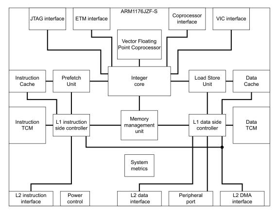
Figure 1-1 ARM1176JZF-S processor block diagram
