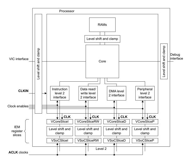
Figure 9-3 Processor clocks with IEM
