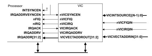
Figure 12-1 Connection of a VIC to the processor
