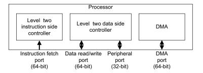
Figure 8-1 Level two interconnect interfaces
