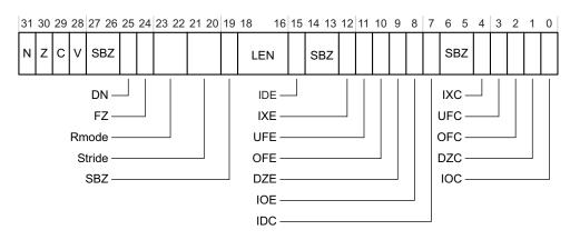
Figure 20-6 Floating-Point Status and Control Register
