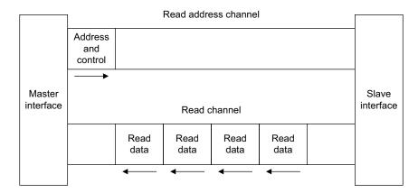
Figure 8-2 Channel architecture of reads
