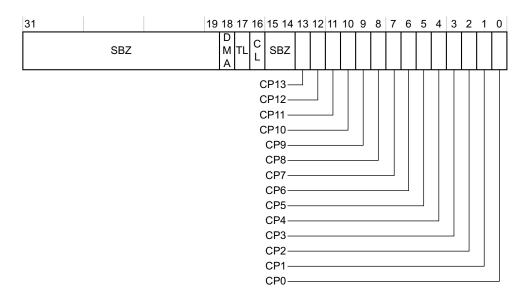
Figure 3-31 Non-Secure Access Control Register format
