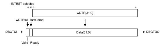
Figure 14-11 Scan chain 5 bit order, INTEST selected
