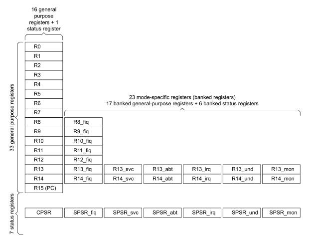
Figure 2-7 Processor core register set showing banked registers
