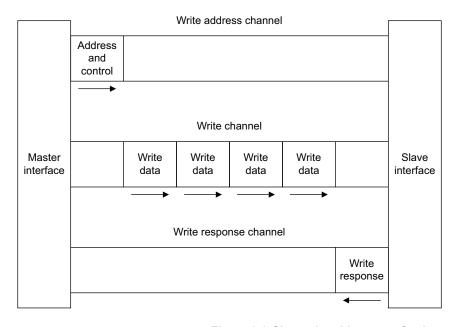
Figure 8-3 Channel architecture of writes
