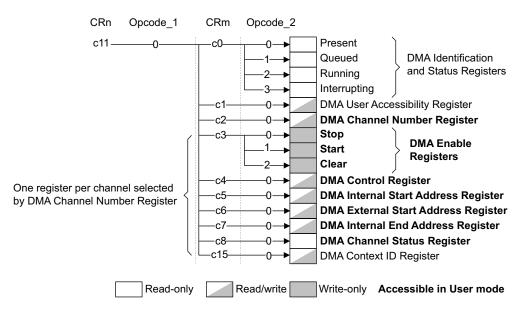
Figure 3-6 DMA control and configuration registers
