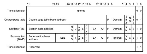
Figure 6-7 ARMv6 first-level descriptor formats with subpages disabled
