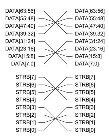
Figure 8-4 Swizzling of data and strobes in BE-32 big-endian configuration
