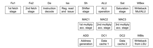
Figure 1-2 ARM1176JZF-S pipeline stages
