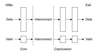
Figure 11-10 Load data buffering
