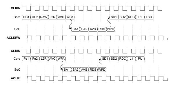
Figure 9-5 Read latency with IEM
