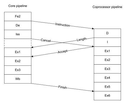
Figure 11-1 Core and coprocessor pipelines
