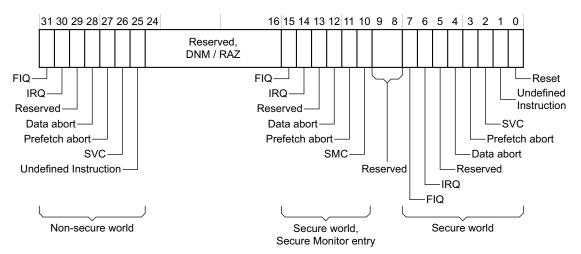
Figure 13-5 Vector Catch Register format
